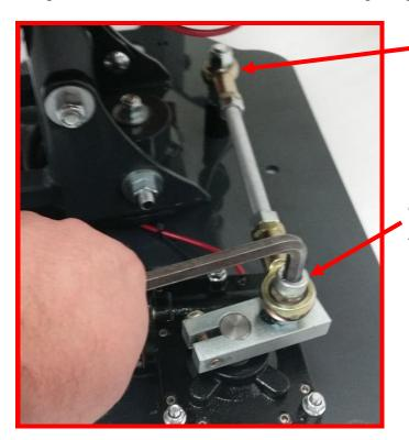
REMOVE THIS END TO ADJUST THE THREADED ROD LENGTH IF NECESSARY!
