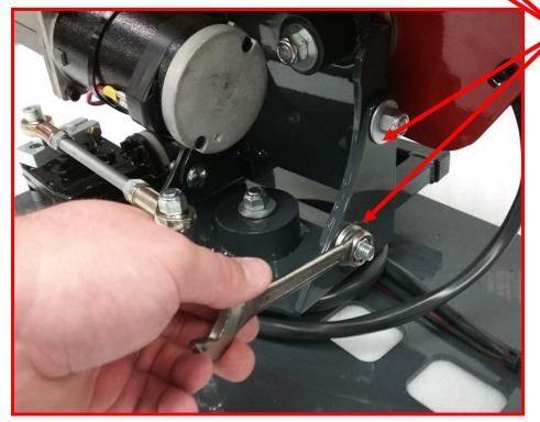
LOOSEN/TIGHTEN THIS NUT TO MAKE YOUR TILT ADJUSTMENTS.
