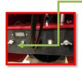
2. 60amp or 70amp relay. Found inside the electrical box. (automotive type)
